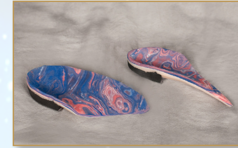
Gait Plate – 3mm High Density Polyethylene shell with an extrinsic rear foot posting and intrinsic forefoot posting. Includes 1/8" Poly-U Cellular Urethane from heel to toes with a choice of Vinyl or Spenco for the top cover. Device is made to control in toeing and out toeing.
