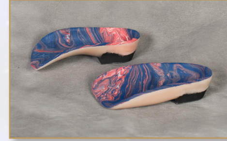
UCBL – 3mm High Density Polyethylene shell with an extrinsic rear foot posting and intrinsic forefoot posting. Includes an EVA top cover to met heads. Device is made rigid with high medial and lateral flanges.
