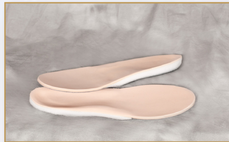
Diabetic – White Plastazote® shell with intrinsic rear foot and forefoot posting. Includes 1/8" Poly-U Cellular Urethane from heel to toes a Plastazote® top cover. Device is used for ultra-flexible control levels.
