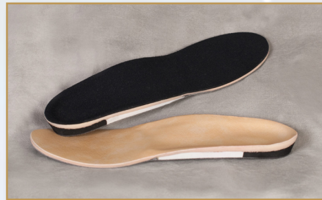
Rigid – 4mm High Density Polyethylene shell with an extrinsic rear foot posting and intrinsic forefoot posting. Includes 1/8" Poly-U Cellular Urethane from heel to toes with a Neolon top cover. Device is used for semi-rigid to rigid control levels. Shown with optional arch fill.
