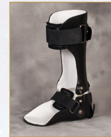
Hinged AFO – Our Hinged AFO is designed to allow range of motion of the ankle joint through the use of an ankle hinge. Includes a choice of plastic shell materials (Polypropylene and Co-Polymer) with varying thicknesses. Also includes a Durafoam liner with choice of thickness for cushioning and comfort.
