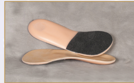
Dress – 2mm High Density Polyethylene shell with intrinsic rear foot and forefoot posting. Includes 1/8" Poly-U Cellular Urethane extension to sulcus with a Vinyl top cover. Device is used for flexible to semi-rigid control levels.
